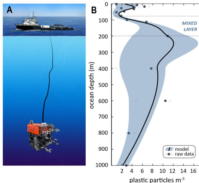
Using MBARI's underwater robots, equipped with sampling devices designed specifically for this project, the researchers filtered plastic particles out of seawater on multiple occasions at two different locations and at various depths--from five to 1,000 meters below the surface of Monterey Bay, California. Some samples were collected just offshore of Moss Landing Harbor, but the majority were collected about 25 kilometers from shore, in the deep waters of Monterey Canyon.
